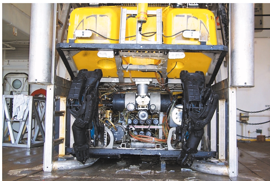
Figure 2. The front of the Oceaneering ROV in its aluminum holding cage on deck. Black manipulating arms can be clearly seen. This picture does not capture the grace and power of the ROV as it moves underwater, autonomous save for its telemetry umbilical.
